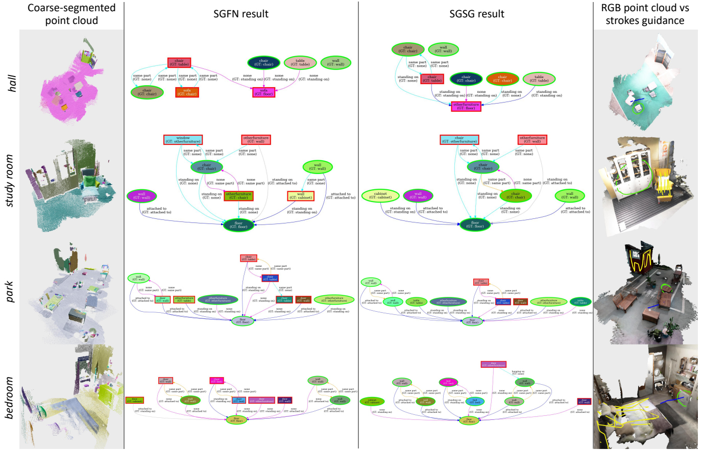
Fig. 6: Comparison of SGFN [39] and our SGSG on Segm-I20. The first column shows the input coarse-segmented point cloud, and the fourth column adds the interactive strokes guidance for SGSG. The second and third columns display SGFN and SGSG results, with correctly predicted nodes circled in ○ and incorrectly predicted nodes framed in □ . Node background color corresponds to coarse-segmentation pseudocolor. For predicates, correctly predicted edges are marked with → , and “same part” edges are highlighted with → . Incorrectly predicted edges are marked with → , and those falsely predicted as “none” are marked with → . Generically predicted edges not annotated in the dataset are marked with → .
