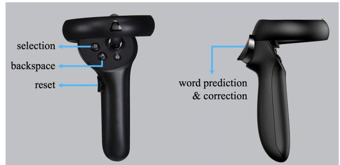
Fig. 3: The functional buttons on the controller used in our method.
