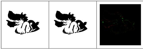
**Fig. 7** Dragon scene with 1 light rendered with ray tracing (left) and our method (middle). The approximation errors of our method are 0.4% (right). Pixels where the images are too bright/too dark are shown with red/green
