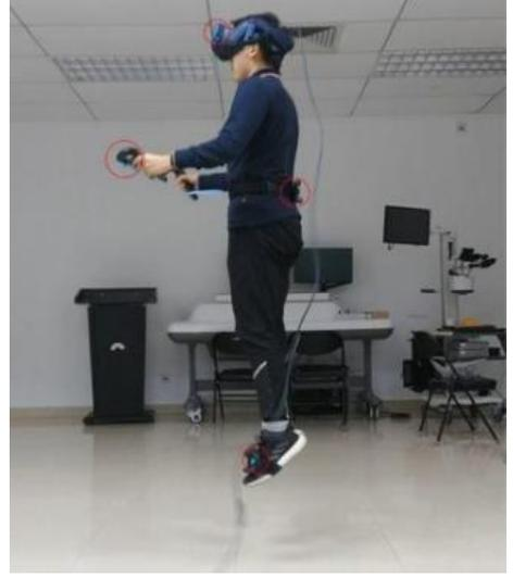
**Figure 1** Experimental setup: An HMD, two controllers, and three trackers.
